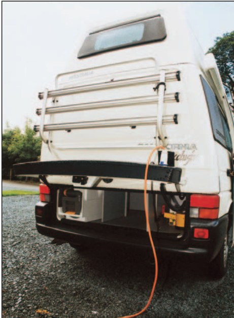
No tailgate, but a small opening flap across the rear of the Westfalia for loading long loads and servicing the loo (left of photo). Bike rack was one of the options fitted to test vehicle.
