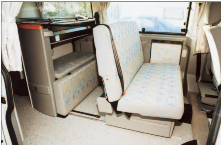
First stage of bed-making is to slide the rear seat forward. Behind it you can now see the cushion under the kitchen that makes the feet end of the bed and the vertically stored cushion that hinges up to complete the bed once the seat is flattened.
