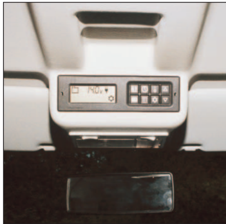
Above the interior mirror is this control panel for fridge and heating; battery and water levels are also displayed.
