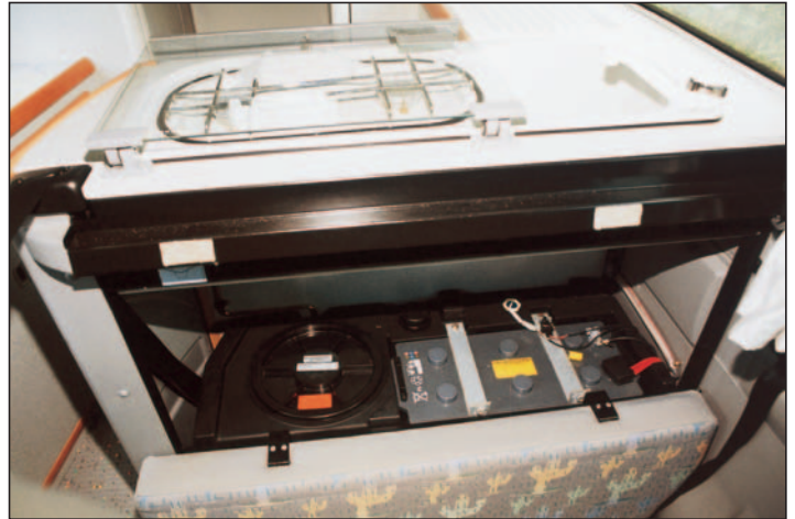
Under the kitchen (with cushion removed) you can see the gas locker (left) and auxiliary battery (right). Waste water tank is also here.
