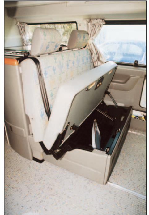
Stowage space is available under the rear seat. The squab tips up for access and is supported by a strut.
