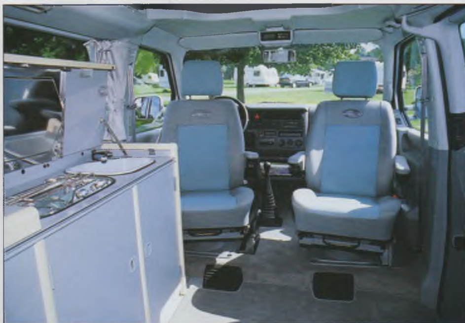
Both cab seats swivel to integrate the cab into the living area. Heater ducts can be seen at floor level
