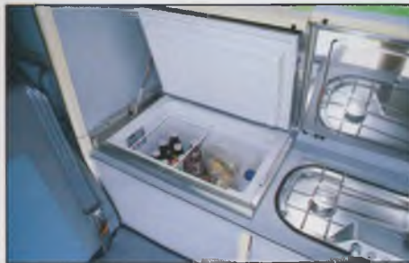
Top-loading compressor-type fridge has only 40-litre capacity, but is ideal for this size of camper
